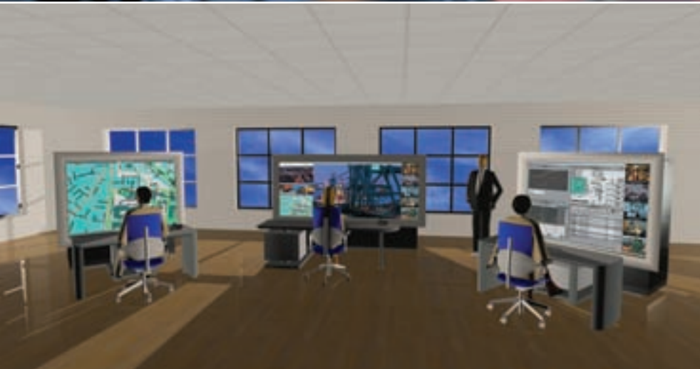
Personal walls: doing away with a clutter of equipment from multiple computers for different functional systems and different display technologies
