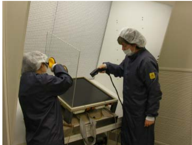
Front bonding of a rugged LCD display for improved optical performance
