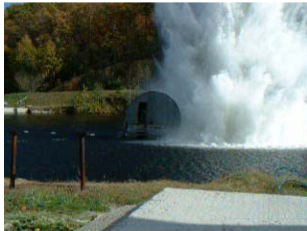
Mil-S-901D Heavyweight Shock Testing with explosive charges
