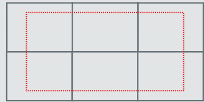
One video source can overlap multiple screens in a video wall.
